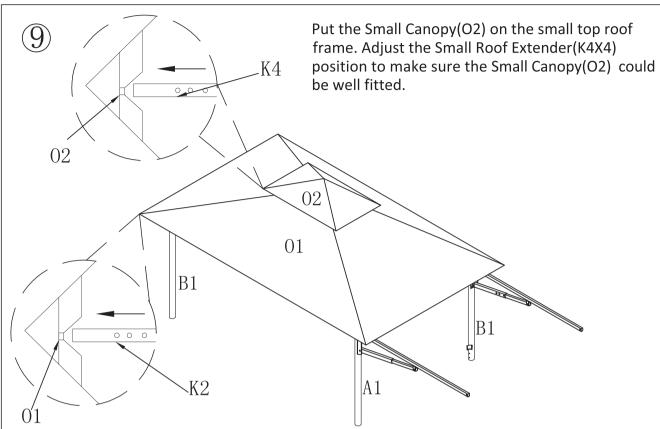
Adjust the Big Roof Extender(K2X4) position to make sure the Big Canopy(O1) could be well fitted.
