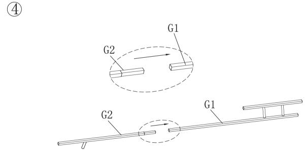
Connect the Upper Roof Frame Bars(G1x4) and the Lower Roof Frame Bars(G2x4).
