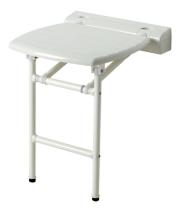
Folding Shower Seat with support legs, manufactured from ABS plastic and structurally re-enforced with steel tubing to give it strength and rigidity. Internal friction plates operate the seats lowering and raising of the legs safely and preventing crashing down on your feet. The design uses very little space when in the up position. The support legs have 25mm adjustment for
