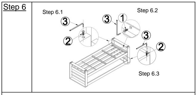
**6.1)** Attach Right Side Panel(B) to Seat Panel(C) using Bolts(2) with Allen Key(3) as shown above.
