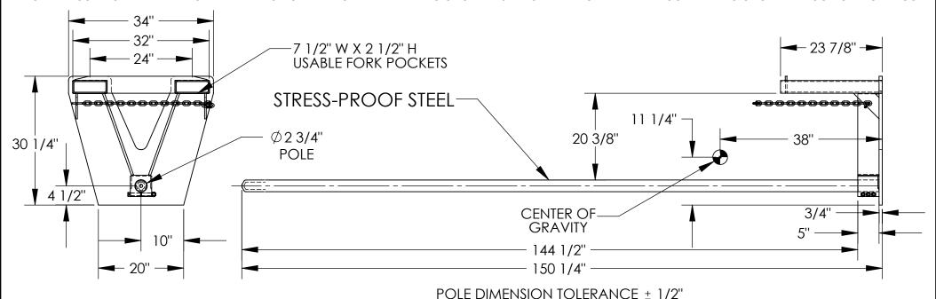
HORIZONTAL CENTER OF GRAVITY: 38" VERTICAL CENTER OF GRAVITY: 11 1/4" LOST LOAD: 520 LBS. (APPROX.)
