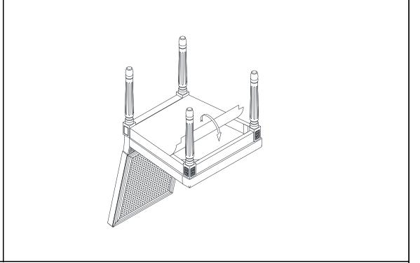
Place the Seat Base Cover back as shown in picture. Smooth the Magic Tape down, Make sure all parts are connected and securely locked into position.
