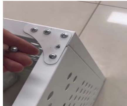
Step 4: In order to stabilize the installation, the triangular connecting piece needs to be installed at the left and right corners at the bottom. Attach two triangular aluminum plates to each of the two corners
