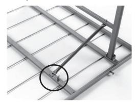
Secure the two pieces by locking the head of the stud into the slot on the opposite base.
