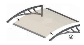
Mount the assemble board on the brackets and connect them with bolt ⑤ and ⑦. (It's recommend to place the board vertically when mounting the brackets.)
