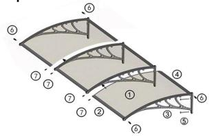
Drill eight holes before installing the canopy. Make sure the holes you drill can exactly match to the holes of the bracket.
