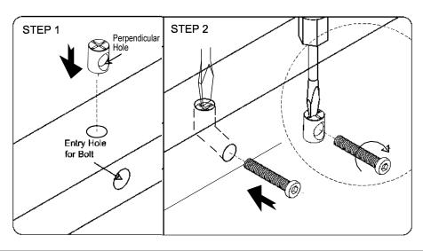
Use a Flat-head Screwdriver to hold Barrel Nut in position before inserting bolt to thread into the Barrel Nut.
