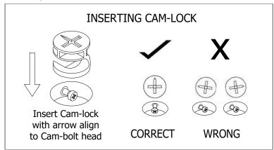
Align the arrow on the Cam-lock to the Cam-bolt head and insert the Cam-lock. Ensure inserted Cam-lock is flushed with the panel.
