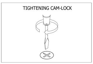
Use a Flat Screwdriver to turn Cam-lock clockwise so it locks onto the head of the Cam-bolt. Turn until it is snug (about one half a turn) -- over-tightening could damage Cam-lock or/and Cam-bolt.
