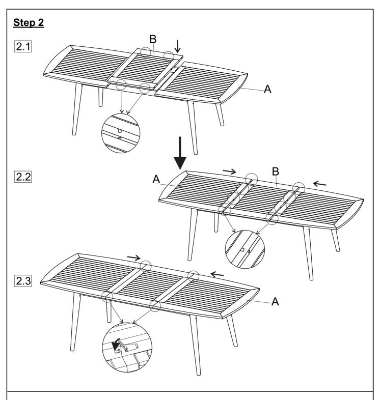
**2.1)** Put the Expansion Board of Table Top(B) in the middle of the Table until the iron pins of Expansion Board of Table Top(B) fits in the housing of Table Top(A).
