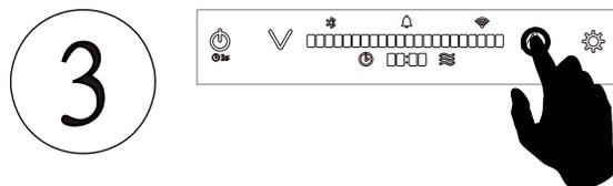
Follow instructions in hood manual to enable the "replace charcoal filter" indicator on the hood controls.
