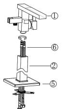
4. Connect the inlet tube like the drawing.
