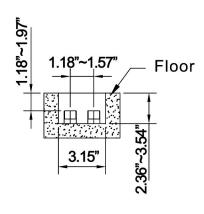
6.Drill holes on floor based on the drawing.
