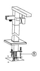
2.Connect the main body with straight tube by screws, by using the screw driver provided.
