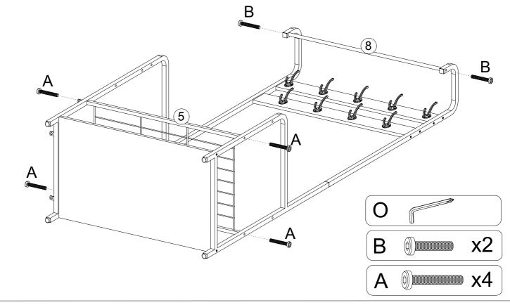
GAUTION: When tightening the screws, tighten sequentially.
