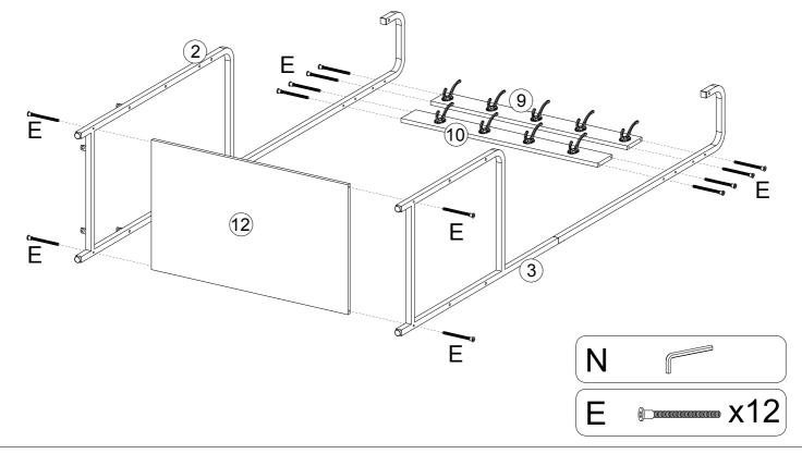
STEP 7 **GAUTION**:When tightening the screws,tighten sequentially.
