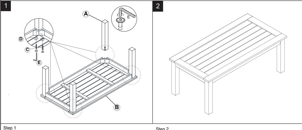
Attach leg frame (A) to Frame Table (B) ,use Bolt (C) and Washer (D) tighten with allen key (E).
