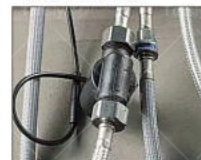
05. Connect the motor to the hose
