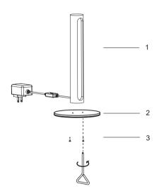
Install the Light Frame (1) to the base (2) until tight through screws (3).
