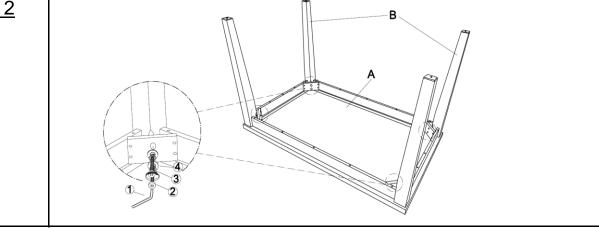
Attach Leg (B) to Top (A) using Bolt ((2)), Spring Washer ((3)) & Washer ((4)) with Allen Wrench ((1)).
