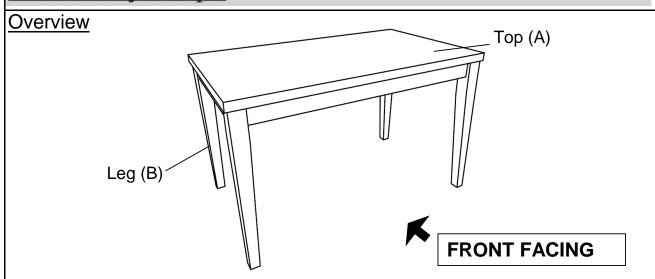
This Counter Height Table has multiple parts and may require up to\_30 minutes to assemble. To give you an overview of the Table parts, the above picture is to help you put the various parts into perspective. Please read through the instructions below to familiarise yourself with the parts and steps before assembly.
