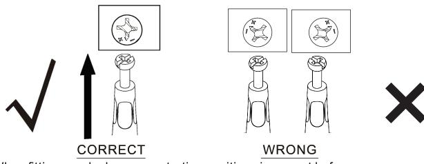
When fitting cam lock, ensure starting positions is correct before you insert cam lock to quickfit.
