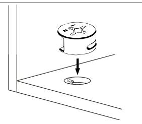
Quickfit head should be in the center of the cam lock. When the two panels are joined. Cam lock should be inserted before quickfit.
