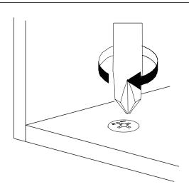
Turn cam lock clockwise to tighten.
