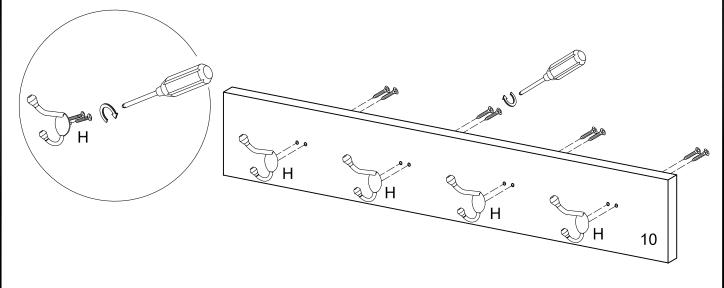
Disassemble screws from hook, then attach hook (H) to part (10) using screw with screwdriver.
