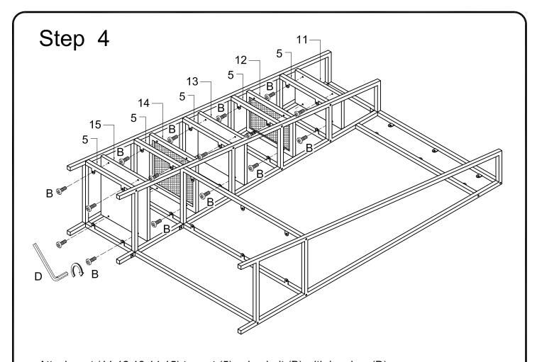
Attach part (11,12,13,14,15) to part (5) using bolt (B) with hex key (D).
