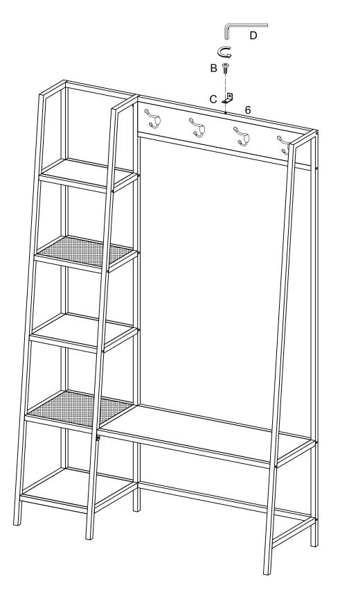
Attach bracket (C) to part (6) using bolt (B) with hex key (D).
