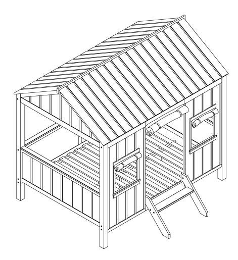
**IMPORTANT**: Do not tighten bolts completely until all bolt are completely lined up and inserted into holes
