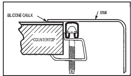
**NOTE:** Do not fully tighten one clip at a time. Partially tighten a clip, then partially tighten the clip across from it. After each clip is partially tightened, repeat the process, fully tightening each clip. This ensures a secure installation and avoids damage to the sink.
