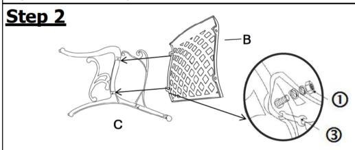
Attach the Chair Seat Panel(B) to the Left Legs with Left Legs with Pre-attached Levellers(C) using Washers, Spring Washers and Nuts(①), with Spanner(③). **DO NOT fully tighten at this stage.**
