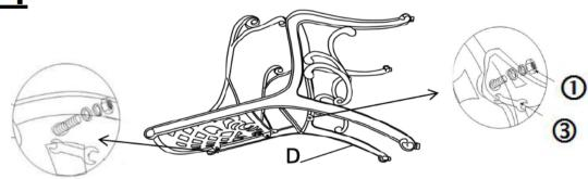
Repeat the same assembly process for the Right Legs with Arm and Preattached Bolts for Seat Panel and Leveller(D)
