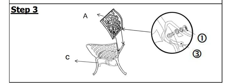
Then attach the Backrest Panel(A) to the top end of the Left Legs with Preattached Levellers(C)using Washers, Spring Washers and Nuts(①) with Spanner(③).
