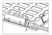
Remove the knock-down hole on box by screwdriver (Part A), Remove screw and take out the driver cover (Part B)
