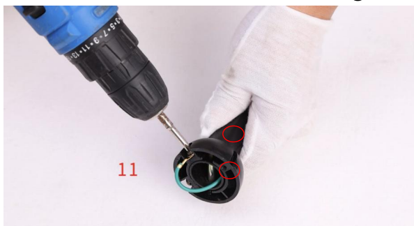
13. Remove 2 screws on the hanger ball
