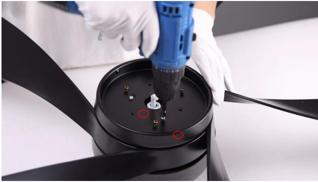
7. Tighten the 3 silver lamp panel screws
