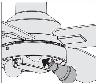
Install the included bulbs into the sockets. When necessary, replace with bulbs of same wattage.
