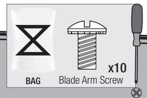
Lightly attach the blade arms to the motor with screws found in the ✕ hardware bag, then securely tighten after both screws are attached.
