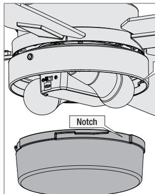
Lift the globe and align the notches in the globe with the tabs in the light kit.
