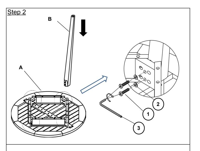
Attach Leg(B) to the Table Top(A) using Bolts( $\widehat{1}$ ), and Washers( $\widehat{3}$ ) with Allen Key( $\widehat{4}$ ). **Do not fully tighten the Bolts.**
