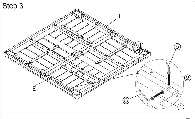
Attach Second Suppor Bars(E) to Foldable Table Top(A) horizontally using Bolts((1)) with Allen Key((5)) and vertically using Bolts((2)) with Allen Key((5)) as pictured above.
