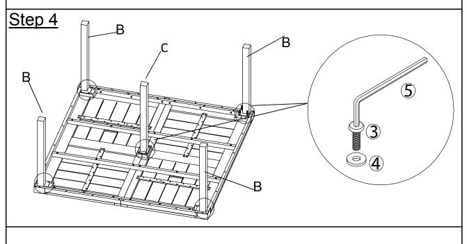
Attach Legs(B) and Support Leg(C) to Foldable Table Top(A) using Bolts(③) and Washers(④) with Allen Key(⑤) as shown in picture above. **Do not fully tighten the Bolts.**
