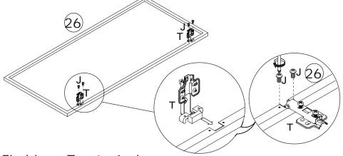
Fix hinge T onto 1 piece board 26 with screw J.
