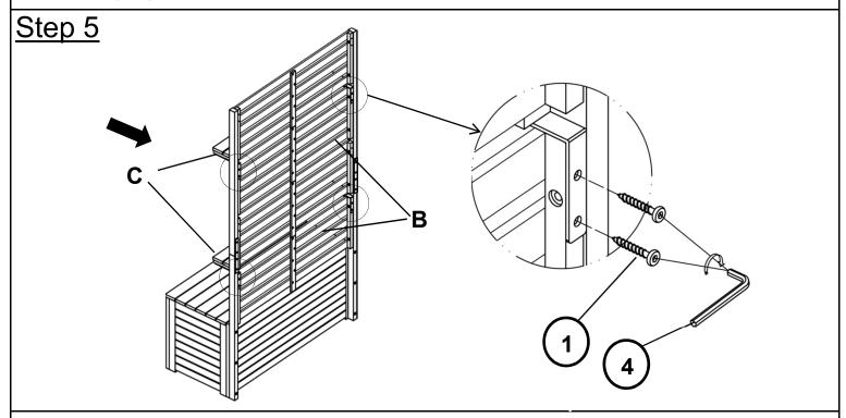
Place the Shelves(C) on the Back Panel(B) as shown above. Attach the Shelves(C) to Back Panel(B) using Screws(1) with Allen Key(4). **Do not fully tighten Screws.**
