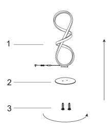
Install the Light Frame (1) to the base (2) until tight through screws (3);
