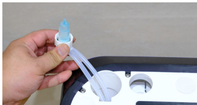
Step 2. Remove the connecting tube of the foam bottle.
