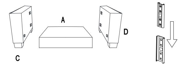
Hook on the Back Frame (B) to Left Panel (C) & Right Panel (D) properly.
