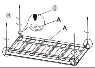
Position the Table Top(A) facedown on a clean, non-marring surface. Insert Iron Bar(⑥) into mounting position at the corner of the Table and tighten with your hand until locked into position.
