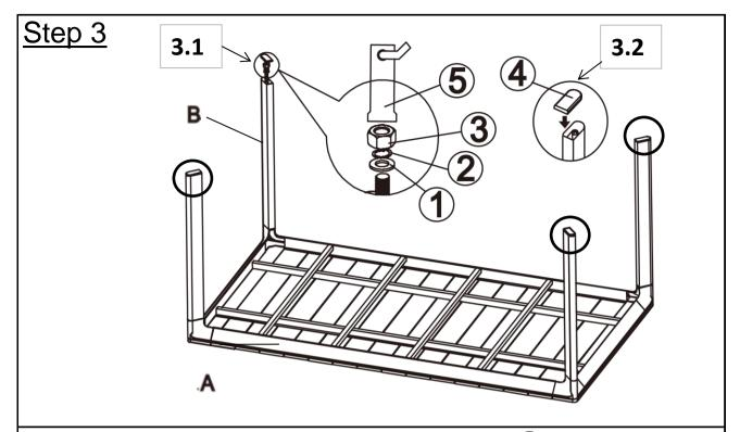
**3.1**Attach Leg(B) to Table Top(A) by placing a Washer(①), Spring Washer(②) and Nut(③) onto the Iron Bar(⑥) and tightening with Socket Wrench(⑤).
