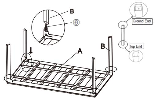
Insert the Leg(B) onto the Iron Bar(6) as pictured above.
