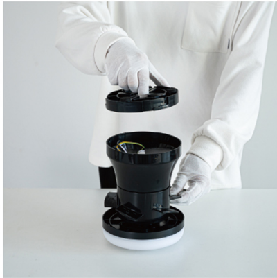
1.Take the cover off the motor
