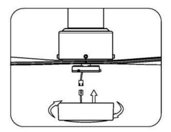
**Note:** Lamping in excess of 75 Watt will disable your light kit. To reset your light kit you must turn the power off and re-lamp keeping the wattage under 75 watts.
