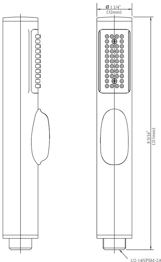
\* Danze Soft Touch Personal Shower is designed to operate only when the button is pressed; water will flow to the spout whenever pressure is released from the button.
