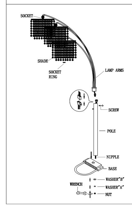
1.SCREW THE NIPPLE WITH LAMP POLE
