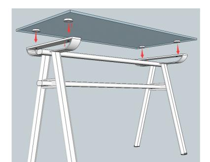
2. Put the screws into the bottom of the frame, and screw it tight.
