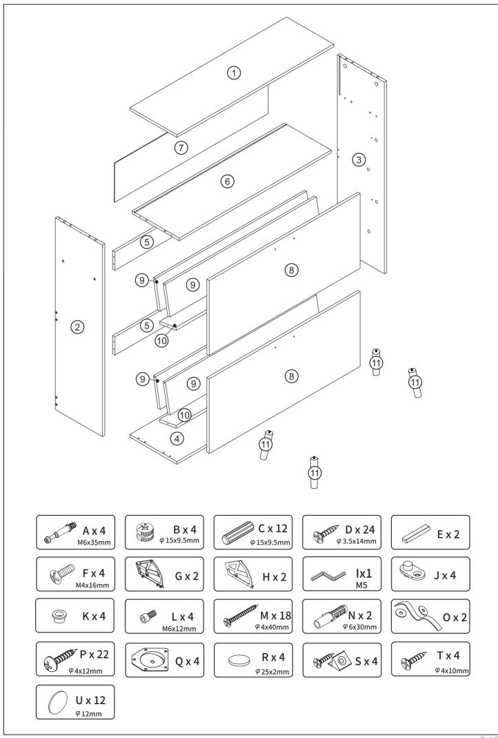
**Step 1** Lock screw (A) on the part ①, then use Hardware (T) to install hardware (J) onto parts ② and ③. The installation position is as shown in the figure below.
