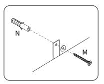
Firstly determine the hole position of the wall, drill holes in the hole position, and insert the expansion screw (N) into the face of the wall. Secondly, place the back of the shoe cabinet against the wall, and install a gasket on theanti-topsy strip and use screw (M) through the gasket and cloth strip to secure the shoe cabinet to the wall.
