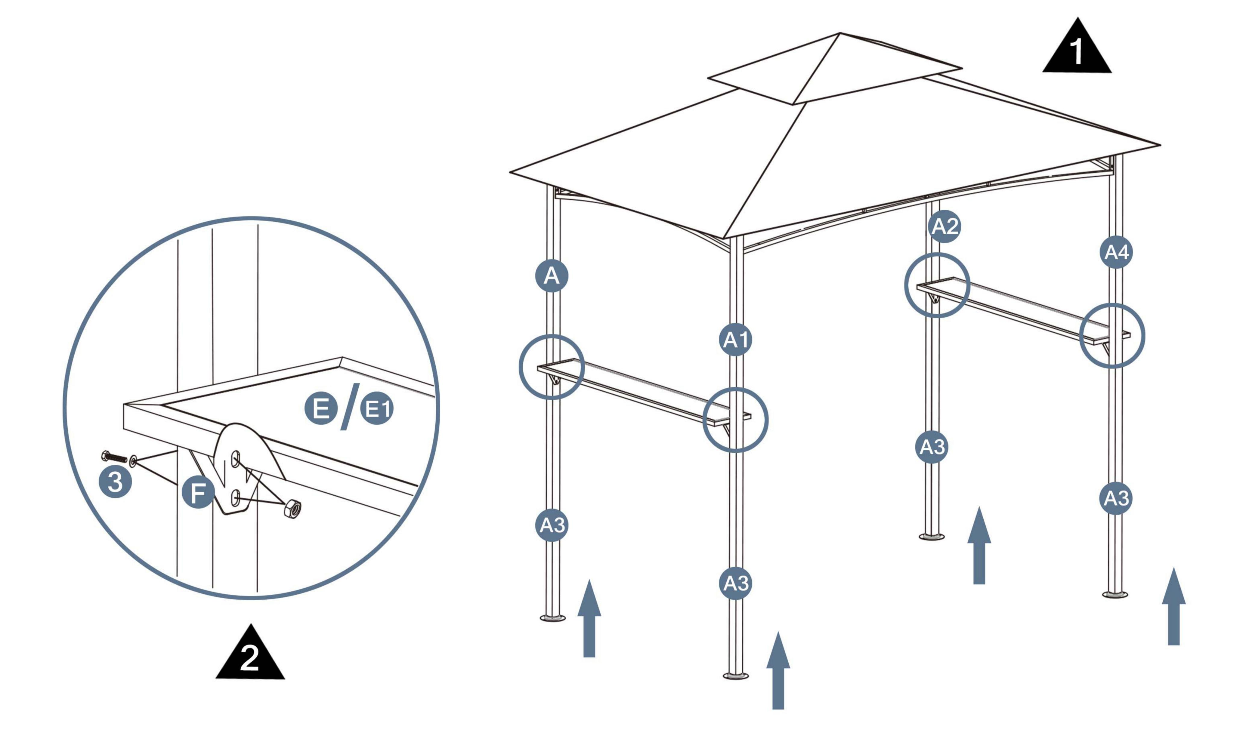
Install the A3 tubes at the four corners first.
