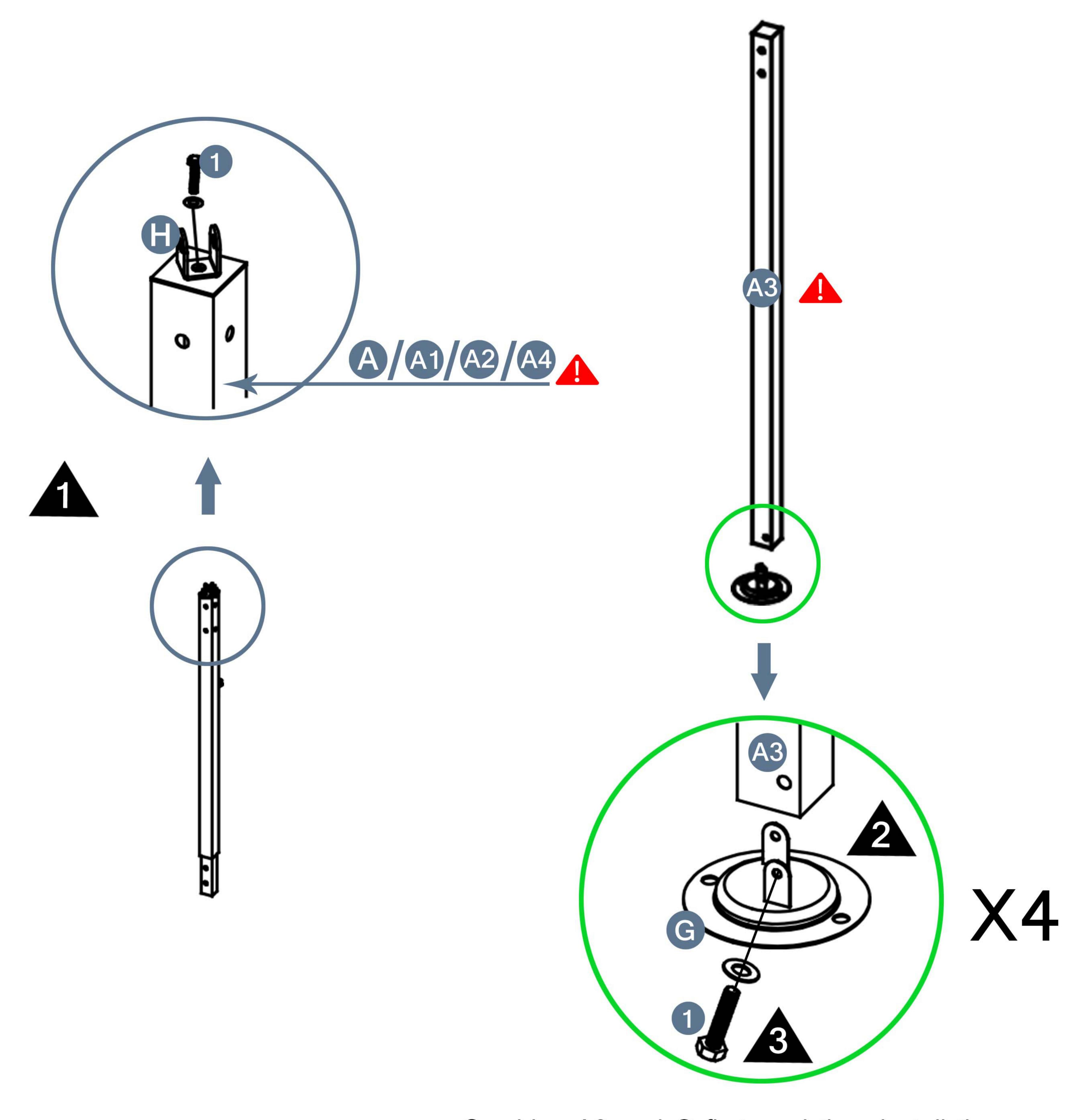
Combine A3 and G first, and then install the screws. In the third step, one screw on each side of the left and right.
