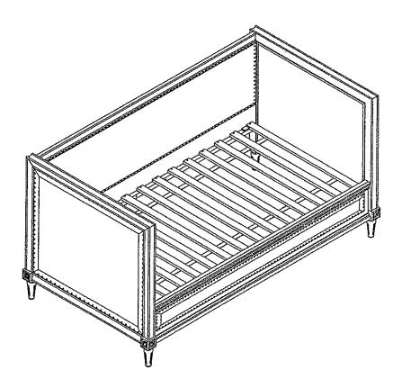
**IMPORTANT**: Do not tighten bolts completely until all bolts are completely lined up and inserted into holes
