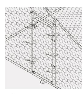
Secure the whole net cover was locked with tie straps
