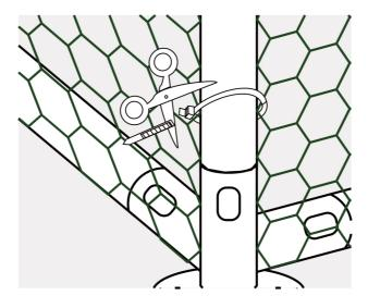
Cut the excess off the cable ties
