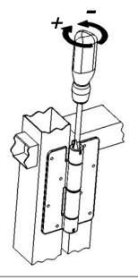
The hinge should be inspected annually, or more frequently if the gate is used often. Spring tension adjustments should be made as needed. The hinge should be regularly lubricated by spraying an oil based lubricant into the area of the cams and barrel.
