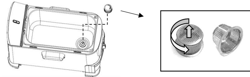
Using a screwdriver or your finger, push the screw located underneath the clean oil container. This will allow the filtration system to open.
