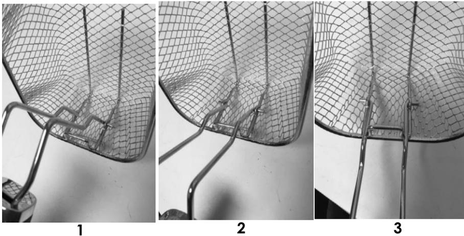
1. Place the pegs into the two holes in the basket bracket. (The pegs are the ends of the two baskets handlebars)
