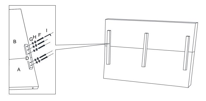
Attached Wooden Leg (C) to the Headboard (A) use Bolt (E), Lock Washer (H) and Flat Washer (G) on both of holes. Turn the Allen Wrench (I) in Bolt (E).
