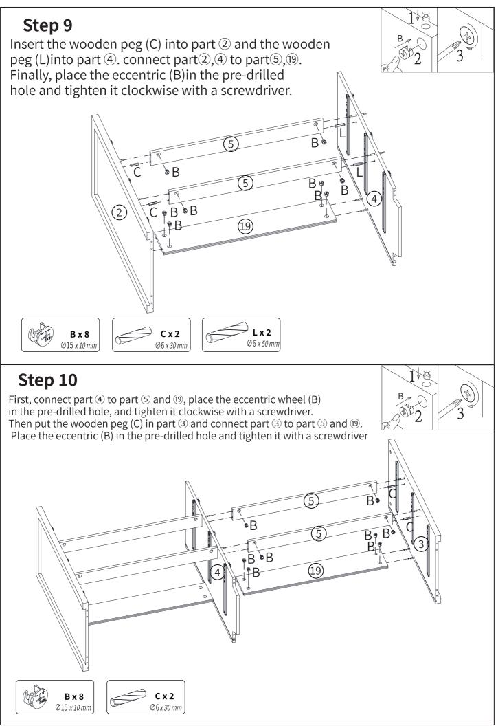
As shown in the figure, part ② is installed along the groove.
