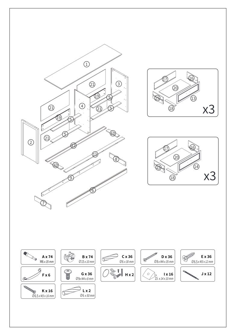
Insert quickfit screws(A) into corresponding holes in part ① ③ ④ as shown.
