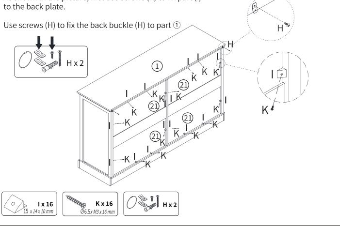
Install (H) in the corresponding position as shown in the figure.
