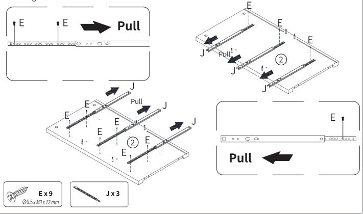
**Step 7** First, align the sliding-rail (J) with the pre-drilled holes on part ③, make sure the arrow on the sliding-rail points in the pulling direction, and then fix it with the two screws (E).
