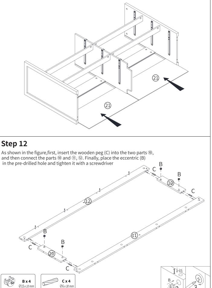
First, place the wooden peg (C) in part (1) and connect parts (9) and (1). Then place the eccentric (B) in the pre-drilled hole and tighten it with a screwdriver.
