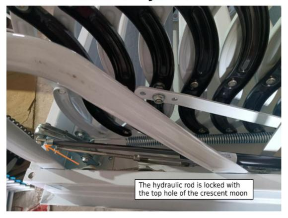
5.Insert the pry bar into the middle of the crescent and the frame, move the crescent upward and insert the screw hole into the second fulcrum hole under the crescent and lock the nut with the fixing screw, and the installation is completed.
