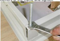
5.Screw on the triangle plate and tighten the nut
