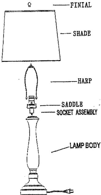
1. FASTEN THE SOCKET ASSEMBLY ONTO THE LAMP BODY. BE CAREFUL NOT TO TWIST THE POWER CORD.
