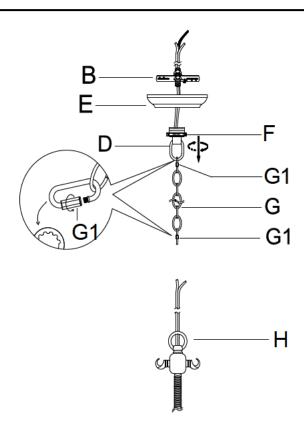
Step 2:Screw the Chain(G) to the Hanging Loop(D) and the loop of the Socket Assembly(H) with Closable link/cap (G1) as diagram.
