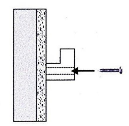
Mount the ledge over the blocks, making sure the groove on the under side of ledge sit tightly into the blocks by tapping ledge downward slightly.
